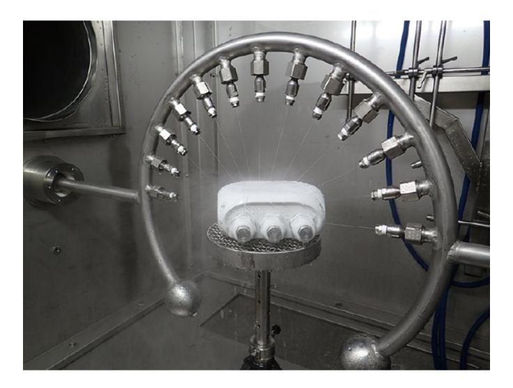
The IP protection class tests are type tests. Prototypes and samples are tested in the laboratory strictly in accordance with the specifications of the desired IP protection class. This involves testing the tightness against the ingress of particles and moisture.
